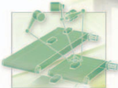
Sistema pick and place mediante robot Delta
